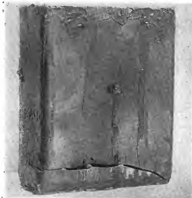
Fig. 17—A cracked battery jar, due to vibration caused by insecure fastening
